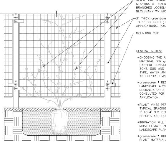
WEAVE VINE BRANCHES INTO SCREEN, STARTING AT BOTTOM. TIE LARGER BRANCHES LOOSELY TO SCREEN, IF NECESSARY W/ BIO-DEGRADEABLE TIES.
